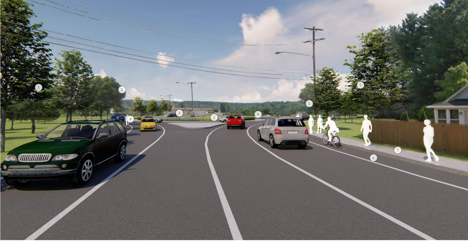
6' BITUMINOUS SIDEWALK (1)WITH GRANITE CURB
